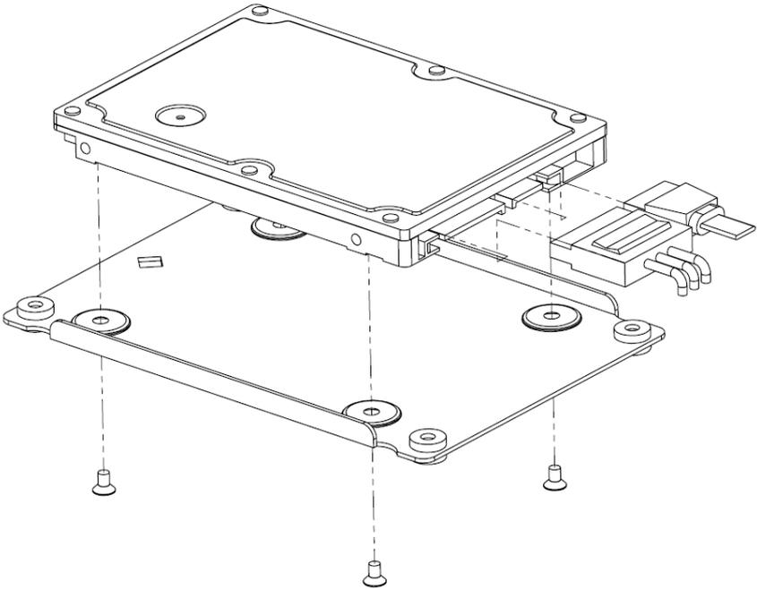
Step 2: Assemble the 2.5" HDD Driver kit with bottom case and connect the SATA signal cable and SATA power cable with the 2.5" SATA HDD Drive.
