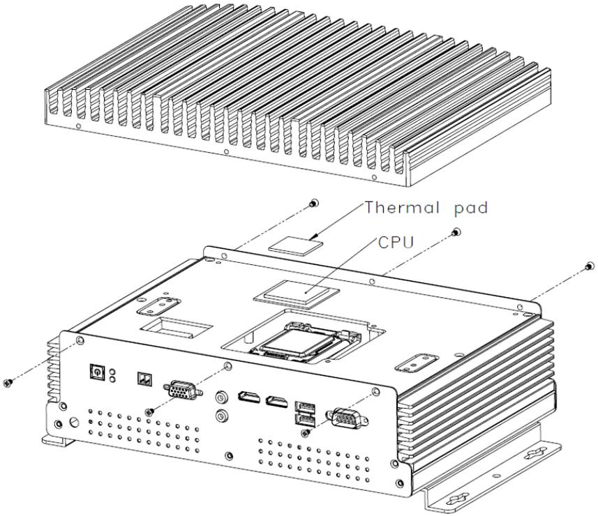
Step 3: Place the heatsink back on and fasten the screws as instructed below.
