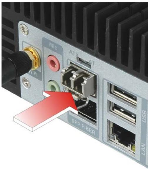
Figure 3-8: SFP Module Installation
