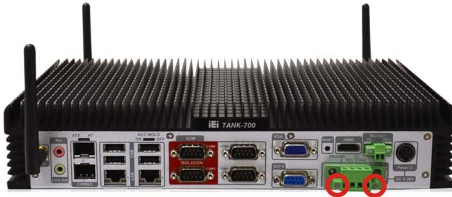
**Figure 3-6: Pluggable DC-in Terminal Block Installation**
