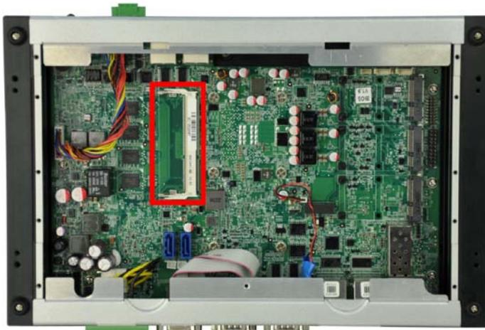
**Figure 3-9: SO-DIMM Socket**
