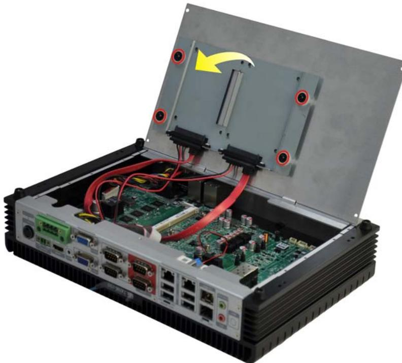
**Figure 3-2: HDD Bracket Retention Screws**
