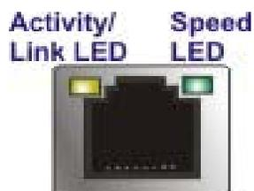
**Figure 3-18: RJ-45 Ethernet Connector**
