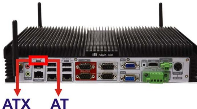
**Figure 3-13: AT/ATX Power Mode Switch**
