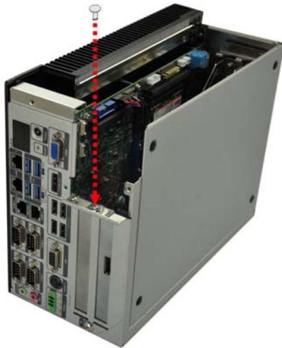
Figure 3-26: Secure iDP Module to System
