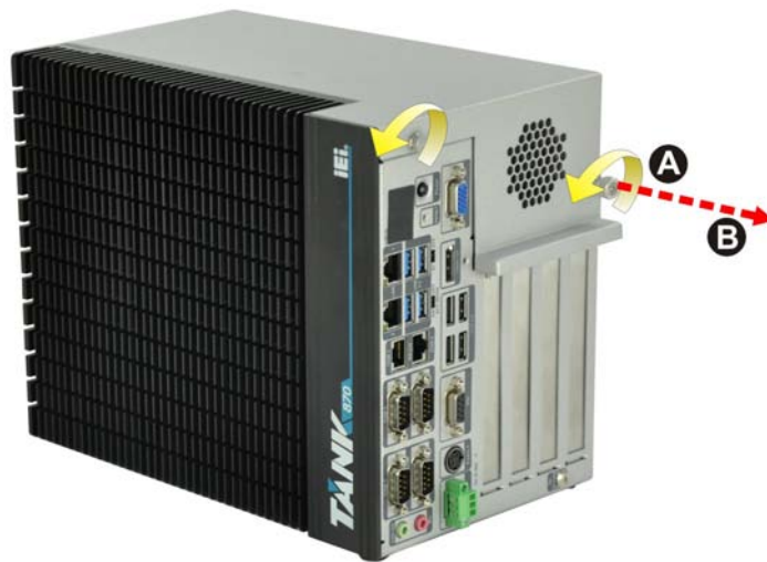
Figure 3-1: Unscrew the Cover
