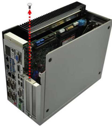
Figure 3-25: Remove Expansion Slot Bracket
