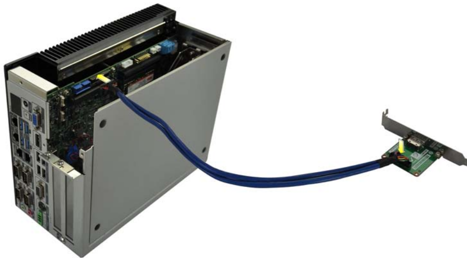
Figure 3-24: iDP Module Installation
