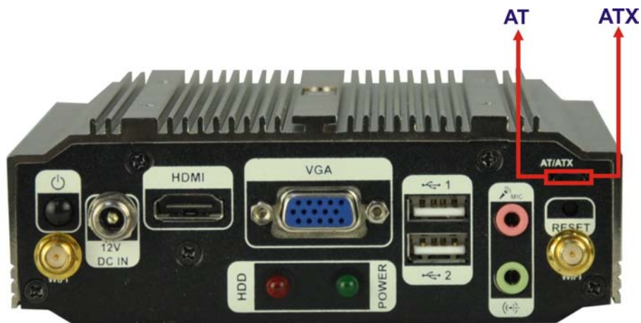
Figure 3-2: AT/ATX Switch Location
