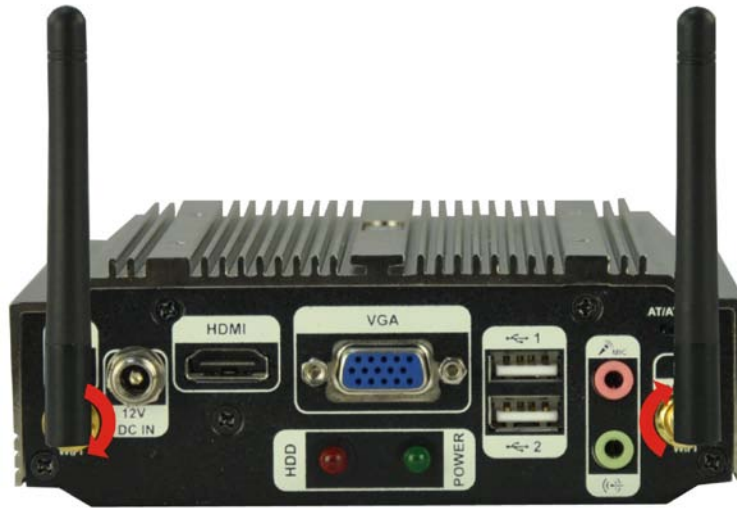
Figure 3-1: Wi-Fi Antenna Installation
