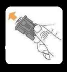
Attach the D-Sub 15-Pin connector to your computer's analog VGA output connector (CNH
