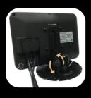
Secure "Tilt" position by adjusting knob
