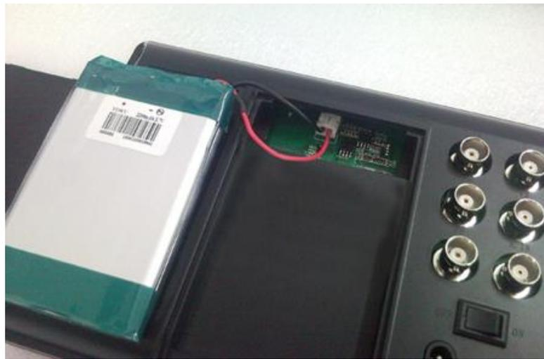
4. Put the battery into slot when check the electricity.
