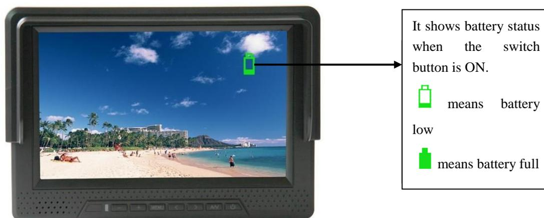
1. Press the switch button to "ON" to start charge, "OFF" to stop charge.
