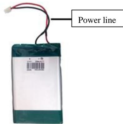
3. Please plug power line into main board's battery socket.
