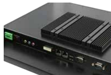
Fan less design, DVI second display output, 12~24VDC power input
