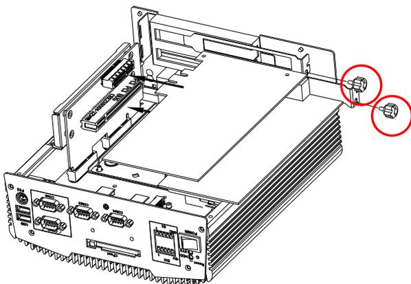
Step 3: Install a hold-down bracket to fix the PCI Card and make sure the PCI Card installs properly. Then, use two screws to fix the hold-down bracket
