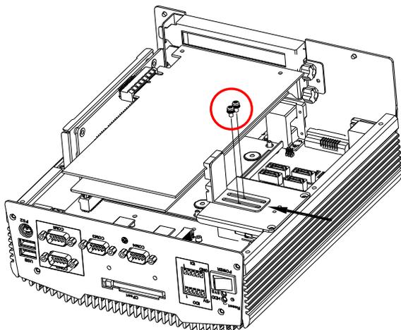
Step 4: Fasten the screws on the front and rear panels, and the brackets of AEC-6967
