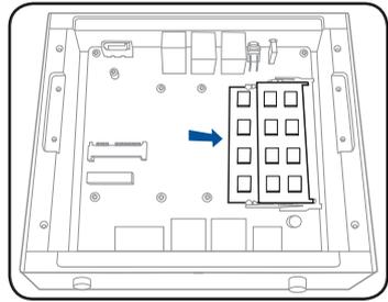
4. Install the Wi-Fi module with half-size mini PCIe interface.
