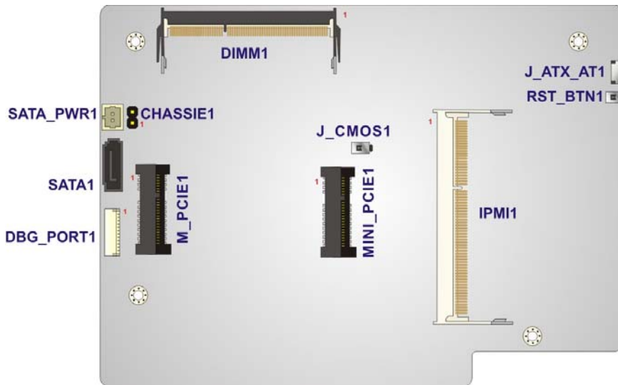
Figure 7-2: Main Board Layout Diagram (Solder Side)
