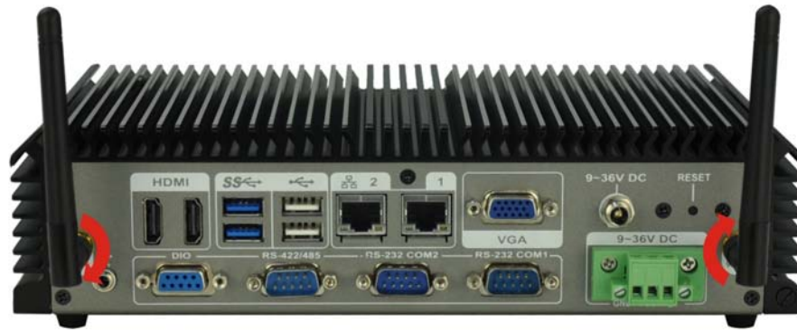
Figure 3-4: Wi-Fi Antenna Installation
