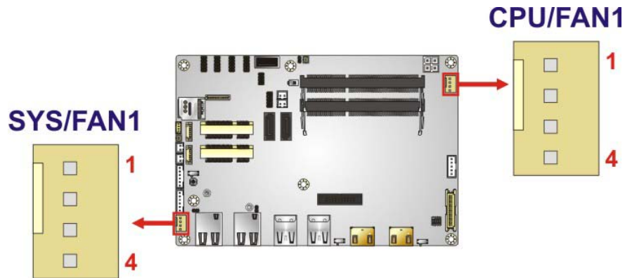
Figure 4-7: Fan Connector Locations
