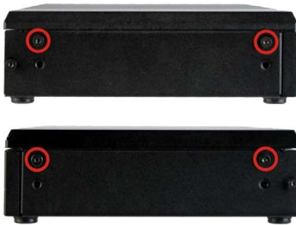
**Figure 5-1: System Cover Retention Screws**
