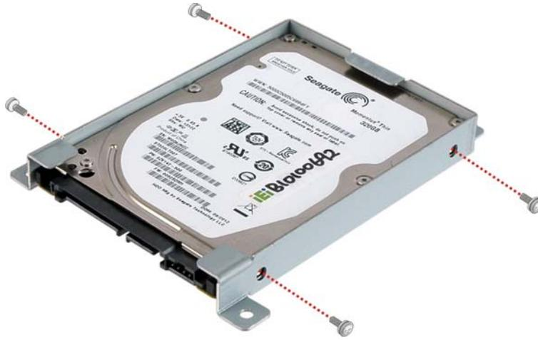
**Figure 3-5:** Inserting the HDD
