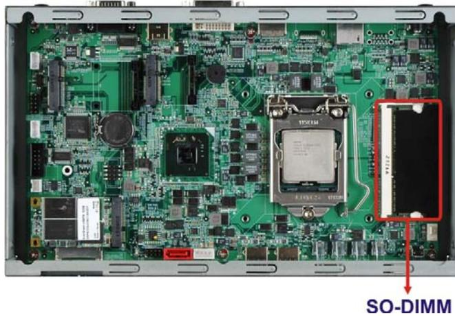
**Figure 5-4: SO-DIMM Removal**
