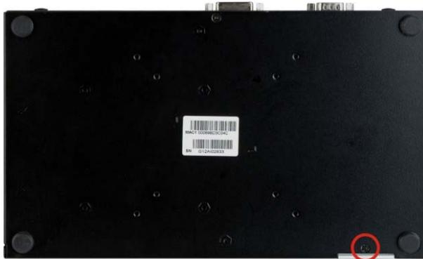
Figure 3-1: SDHC Slot Cover Retention Screw
