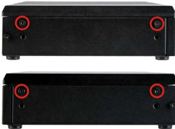
**Figure 3-3: Top Cover Retention Screws**
