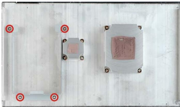
**Figure 3-4: HDD Bracket Retention Screws**
