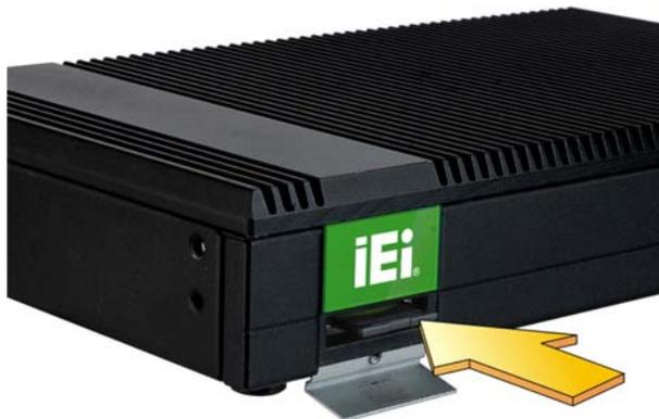
Figure 3-2: SDHC Card Installation
