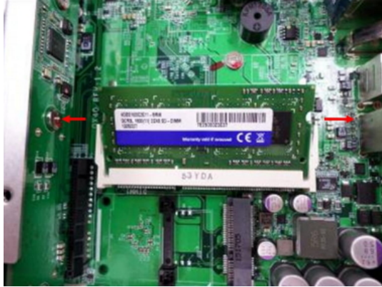
Figure 4-2: Pull the Retention Clips on Each Side
