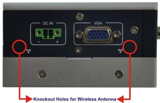
Figure 3-6: Knockout Holes for Wireless Antenna
