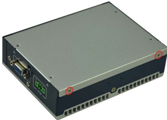
Figure 3-11: Remove the Bottom Panel (ITG-100-AL-E1/S)
