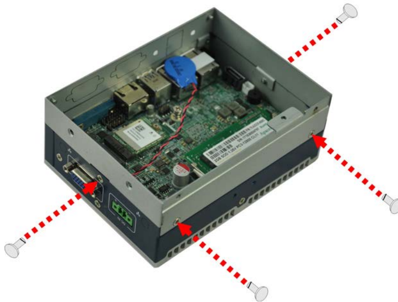
Figure 3-12: Additional Block Layer Installation
