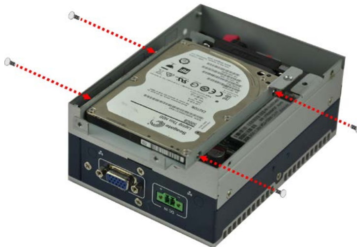
Figure 3-3: Install the HDD
