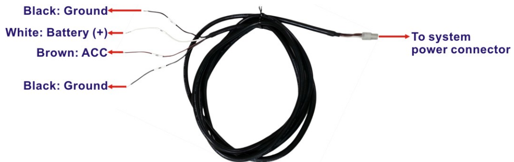
Figure 3-18: ACC Power Cable
