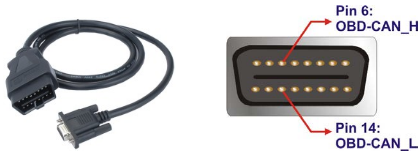
Figure 3-16: OBD-II Cable and Connector Pinouts
