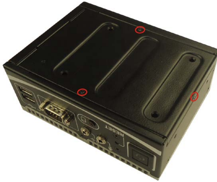
Figure 3-1: Retention Screws Removal
