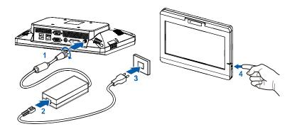
Figure 4 Turning on the system
