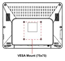
Figure 5 Mounting hole locations on the HPC-1000
