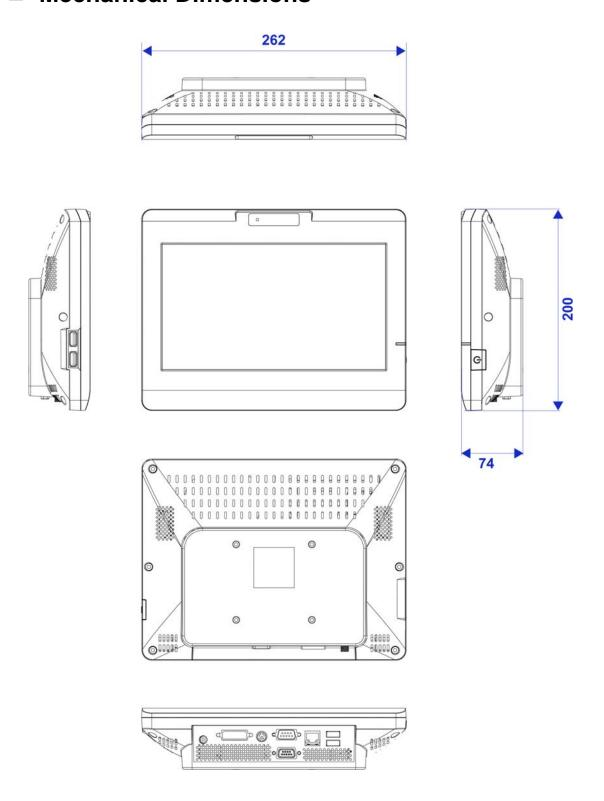
Figure 3 Mechanical Dimensions
