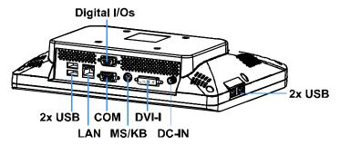
Figure 2 Mechanical Layout - I/O Panel
