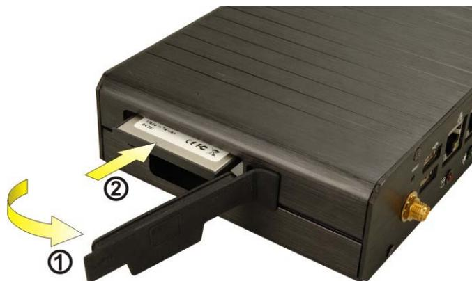
**Figure 4-4: CF Card Installation**
