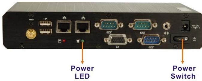
**Figure 4-13: Power Switch and Power LED**
