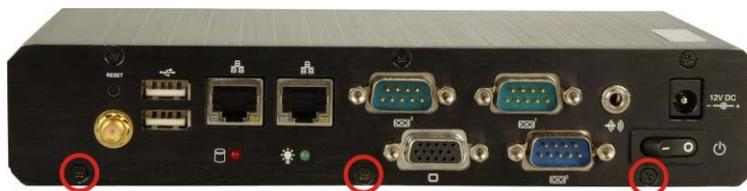
**Figure 4-1: Bottom Cover Retention Screws (Front Panel)**
